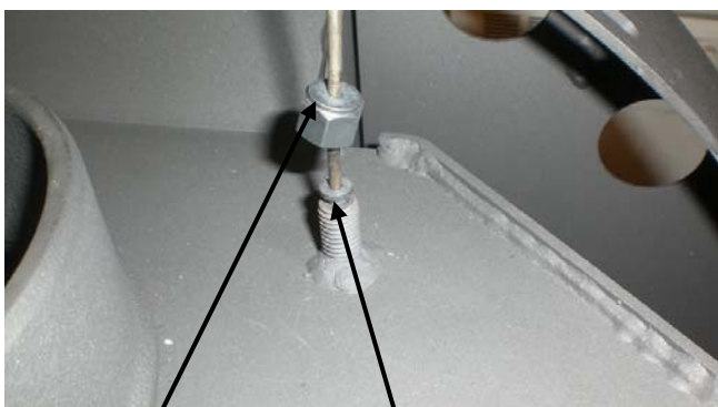
Union nut Sensor sleeve
